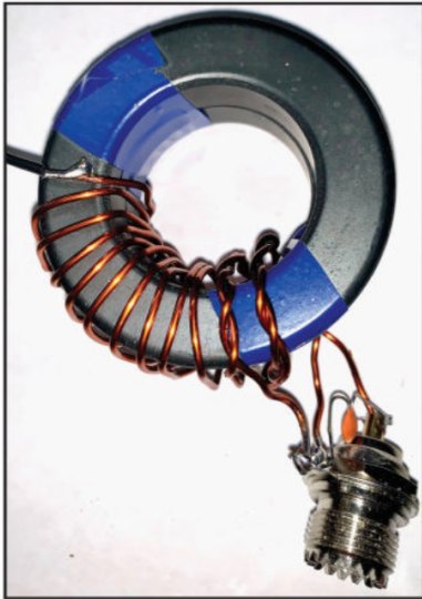
Photo A. Conventional matching transformer for multiband end-fed antenna.
