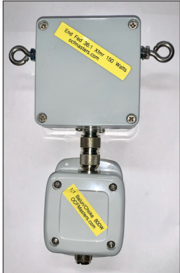
Photo D. Isolation of the transformer from the 1:1 balun in separate boxes coupled together with a dual PL-259 connector to avoid unwanted coupling to the feedline.
